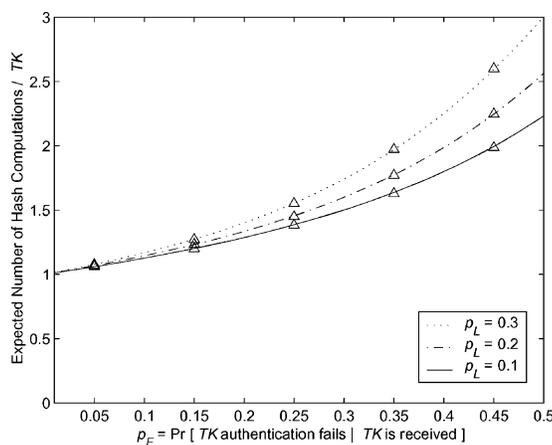
Fig. 11. The expected number of hash computations per TK-disclosure at the client node vs.  $p_F$ :  $p_L = 0.1 \sim 0.3$ ,  $t = 10$ .
