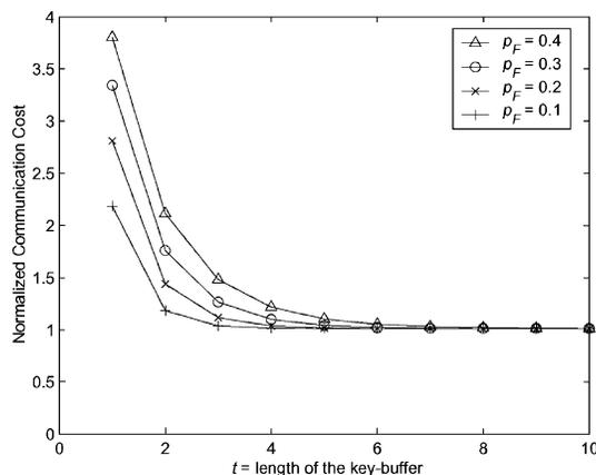
Fig. 12. The normalized communication cost at the client node versus  $t$ :  $p_F = 0.1 - 0.4$ ,  $\alpha = 10$ ,  $p_L = 0.05$ ,  $n = 1,000$ .
