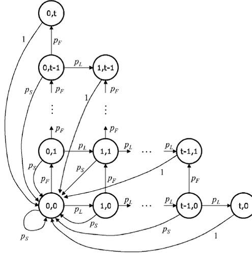
Fig. 13. The state transition diagram for LiSP.
