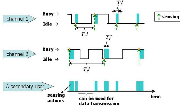
Fig. 3. Periodic sensing of two channels by a secondary user
