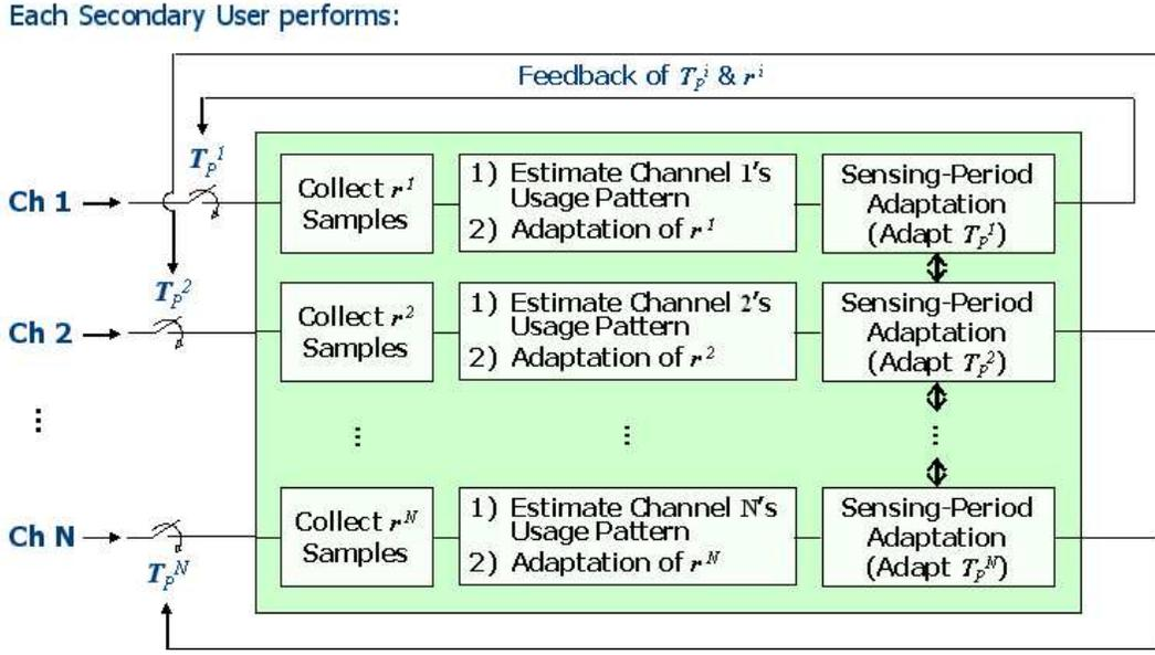
Fig. 4. System diagram of sensing-period adaptation
