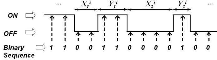
Fig. 2. The ON-OFF channel model
