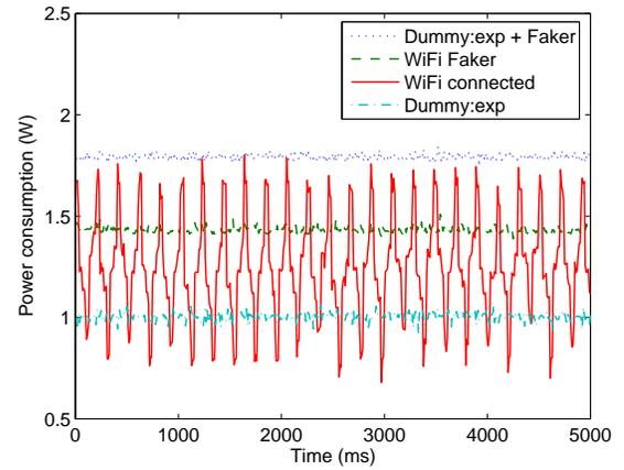
Figure 10: Comparison of the power consumption with WiFi connection, the WiFi faker, and a combination of a dummy program and the WiFi faker. The WiFi device is in power-saving mode in which the WiFi device dozes after every beacon interval.
