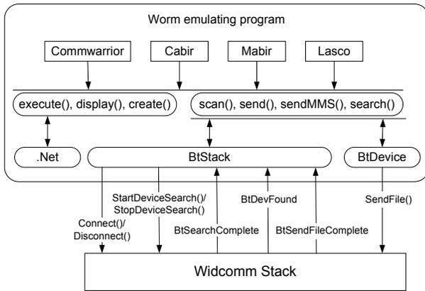
Figure 5: Software architecture of a worm emulator
