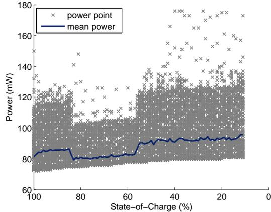
**Figure 6: Power consumption variations with respect to the battery-charge level in software measurement**
