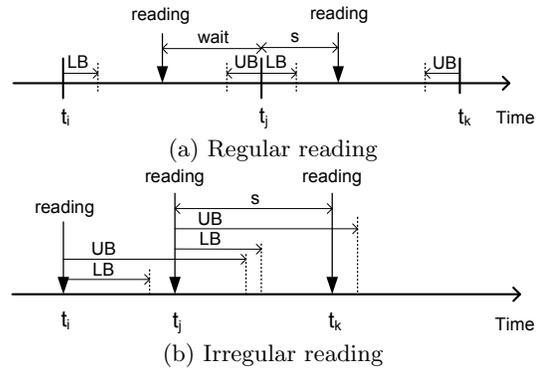
**Figure 3: Power-reading methods: regular reading has a fixed interval based on  $t$ , while irregular reading-points are not fixed. In both cases, reading-points are randomly chosen in between lower bound (LB) and upper bound (UB). A timer object is set to a time period of  $s$ .**
