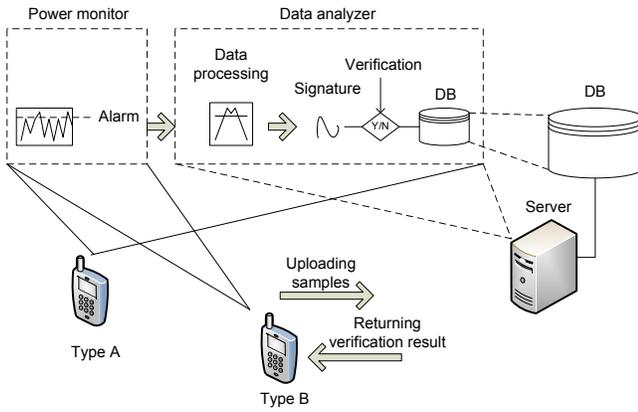
**Figure 2: The system architecture: Type A stands alone and Type B has a remote server/data-sync PC for processing data.**
