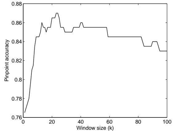
**Figure 8: An optimal window size ( $k$ ) in the moving average filter. When the  $k=23$  or  $24$ , PA is the highest. No compression was applied.**
