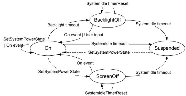
Figure 1: A simplified system power state transition diagram on Windows Mobile OS
