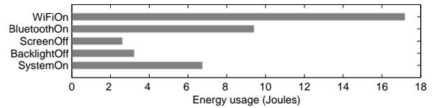
**Figure 4: Energy usage of system states for 10 seconds on the HP iPAQ rx4200. No explicit application is executed in the SystemOn, BacklightOff, and ScreenOff states. For the BluetoothOn and WiFiOn states, the Bluetooth and WiFi radios are turned on exclusively for each state.**
