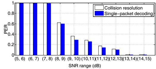
Fig. 6. Comparison between DAC collision resolution and single-packet decoding without collision.
