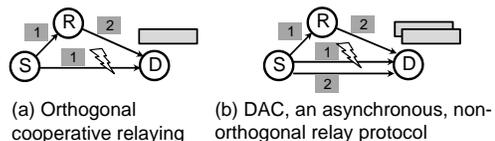
Fig. 1. A contrast between traditional relaying and DAC. The shaded tags denote the order of transmission.
