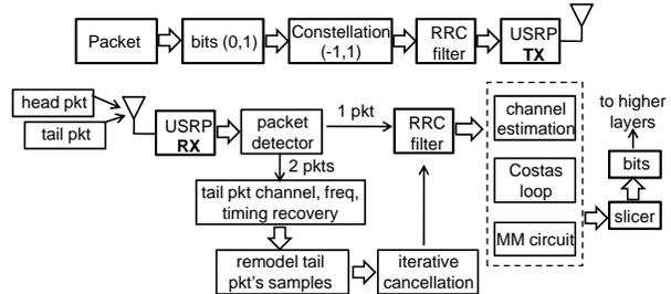
Fig. 3. Flow-chart for DAC transmitter (upper) and receiver (lower).
