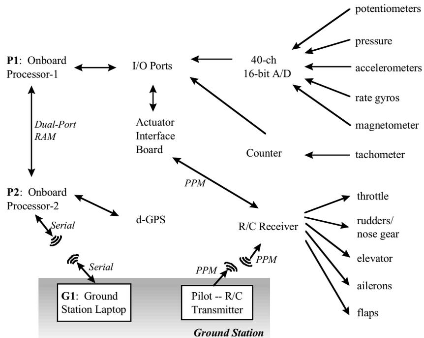
Figure 7-10: UAV Data Acquisition and Communication Systems.
