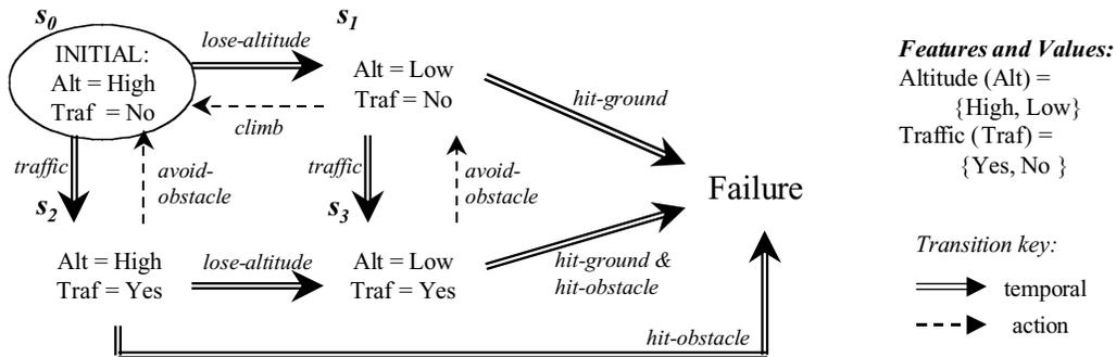
Figure E-1: State-space Example with Multiple Cycles and Dependent *tfts*.
