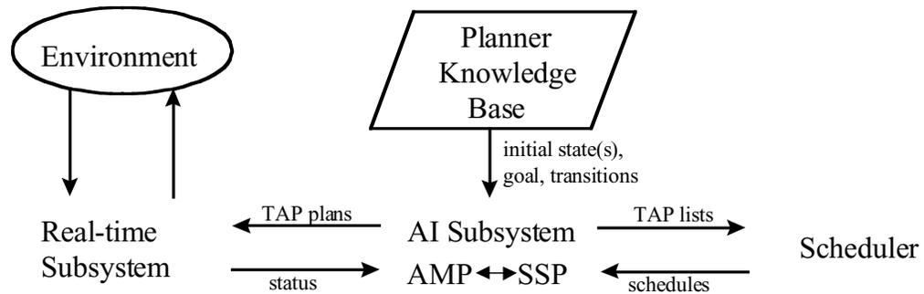
Figure 2-5: The Cooperative Intelligent Real-time Control Architecture.
