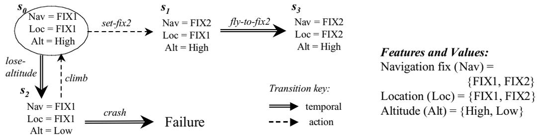
Figure 4-3: Aircraft State-space with a Cycle ( $s_0 - s_2$ ).
