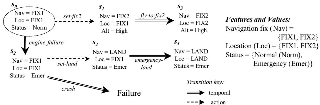
Figure 4-2: Aircraft State-space with Tree Structure.
