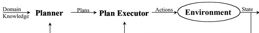
Figure 2-1: A "Generic" Planning/Plan-Execution Architecture.<sup>4</sup>
