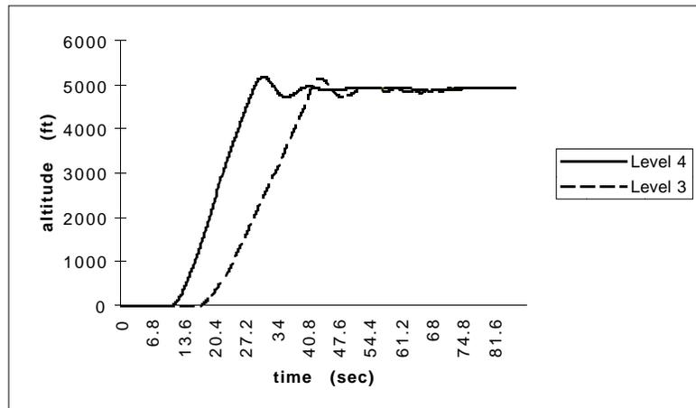
Figure 6-11: Altitude with and without Secondary *Ctrl* Actuation.
