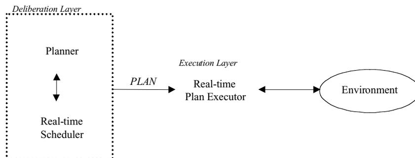
Figure 1-4: Architecture for Generating and Executing Real-time Plans.
