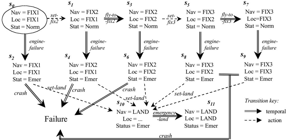
Figure 4-4: Aircraft State-space with a Dependent Temporal Transition (*dt*).
