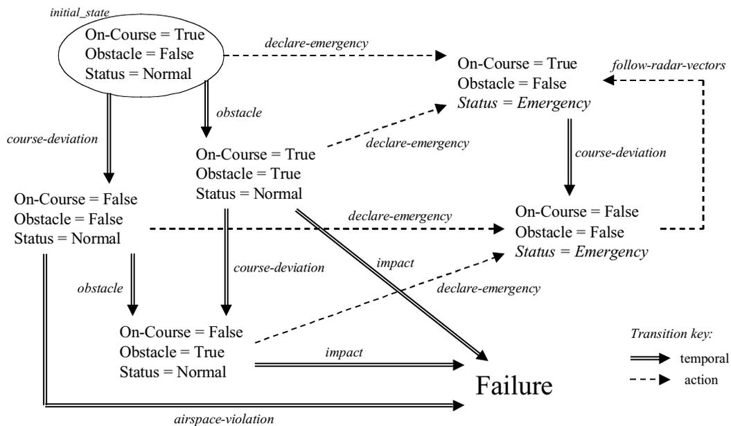
Figure 6-6: Reduced Flight Plan for Failed Processor ( $f_1$ ).
