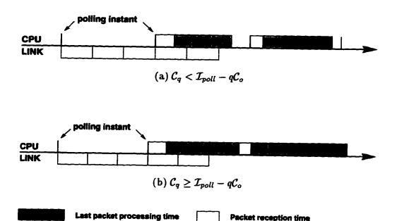
Figure 4.9: Link reception and protocol processing overlap in polled mode input.
