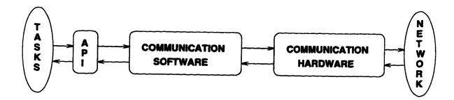
Figure 2.1: Communication subsystem as a pipeline.
