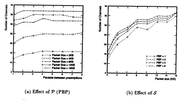
Figure 4.6: Effect of  $\mathcal{P}$  and  $\mathcal{S}$  on channel admissibility in O1.
