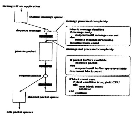
Figure 3.5: Execution profile of a channel handler.
