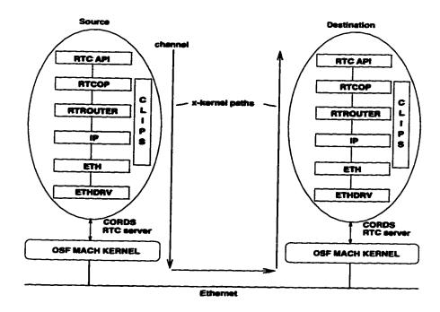
Figure 5.6: CORDS-based service protocol stack.
