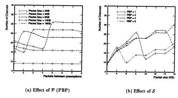
Figure 4.7: Effect of  $\mathcal{P}$  and  $\mathcal{S}$  on channel admissibility in O2.
