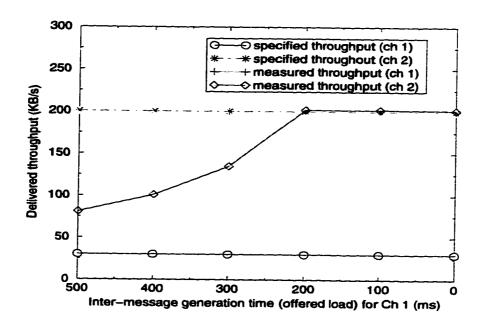
Figure 5.8: Traffic isolation between two real-time channels.
