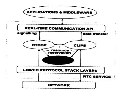
Figure 5.1: Real-time communication service architecture.
