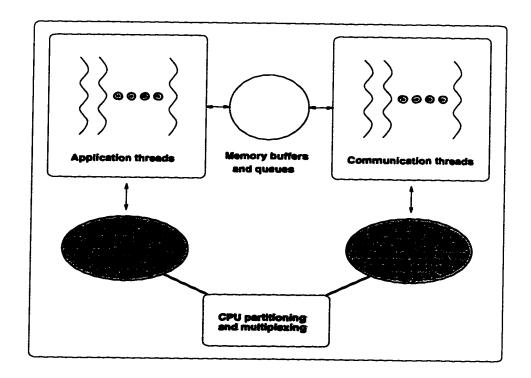
Figure 8.1: Integrated QoS-sensitive computation and communication subsystems.
