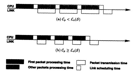
Figure 4.3: Protocol processing and link transmission overlap in O1.
