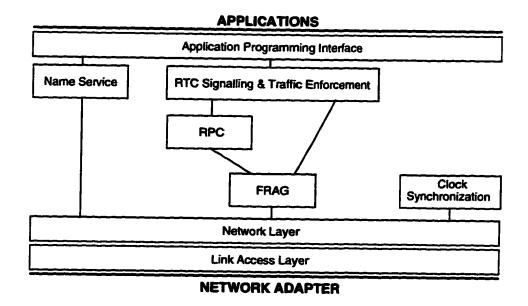
Figure 3.7: Real-time communication protocol stack (x-kernel).
