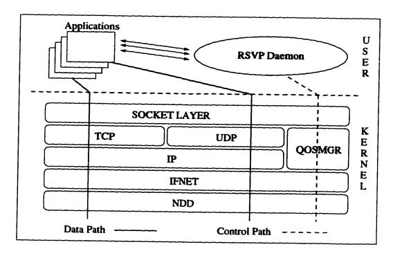
Figure 7.2: Protocol stack architecture and QoS extensions.
