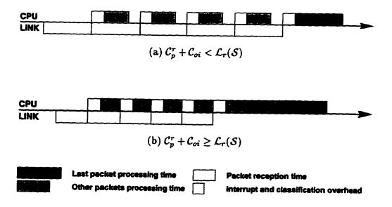
Figure 4.8: Link reception and protocol processing overlap in interrupt mode input.
