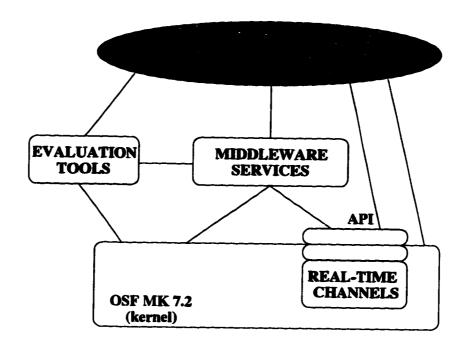
Figure 5.11: ARMADA middleware and real-time communication services.
