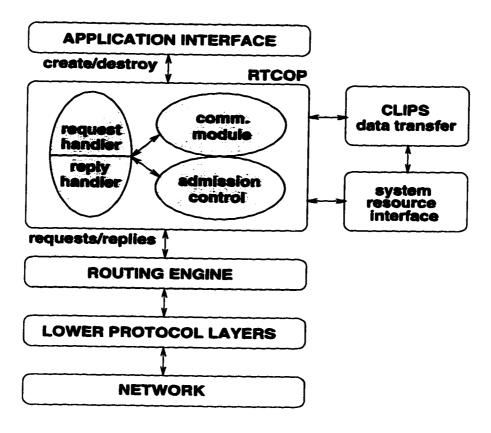
Figure 5.2: RTCOP internal structure and interfaces.
