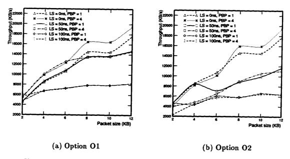
Figure 4.2: Throughput as a function of packet size and link speed.
