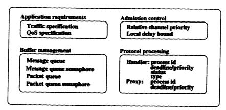
Figure 3.4: Channel state maintained at host.
