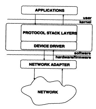
Figure 1.3: Communication subsystem at end hosts.
