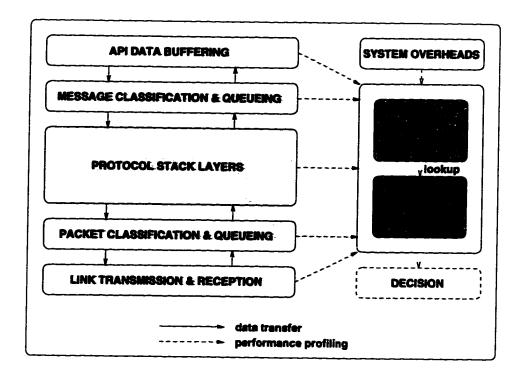
Figure 6.1: Architecture for self-parameterizing protocol stacks.
