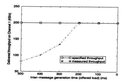
Figure 5.7: Traffic enforcement on a single real-time channel.
