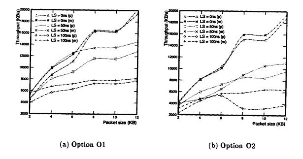
Figure 4.5: Comparison of measured (m) and predicted (p) throughput (P = 4).
