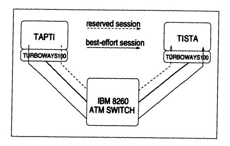
Figure 7.5: Experimental testbed for prototype implementation.
