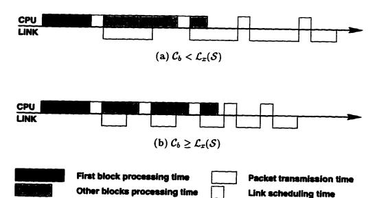
Figure 4.4: Protocol processing and link transmission overlap in O2.
