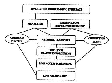
Figure 3.1: Desired overall software architecture.
