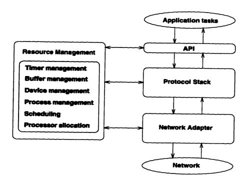
Figure 2.2: Interaction between protocols and resource management functions
