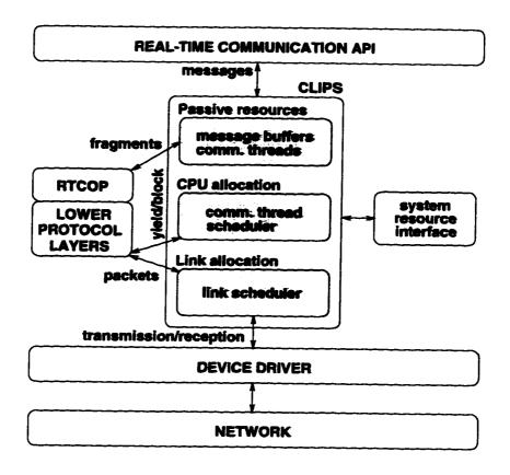
Figure 5.3: CLIPS internal structure and interfaces.
