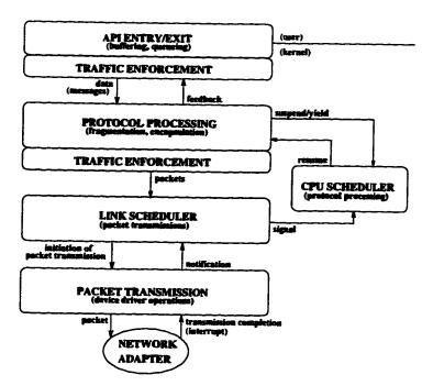
Figure 3.2: Software structure for QoS-sensitive data transmission.
