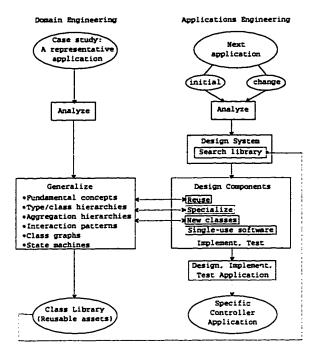
Figure 2.5: Domain model based application development process
