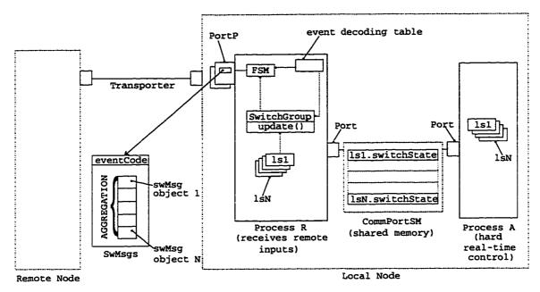
Figure 6.1: Message structuring and handling for efficiency
