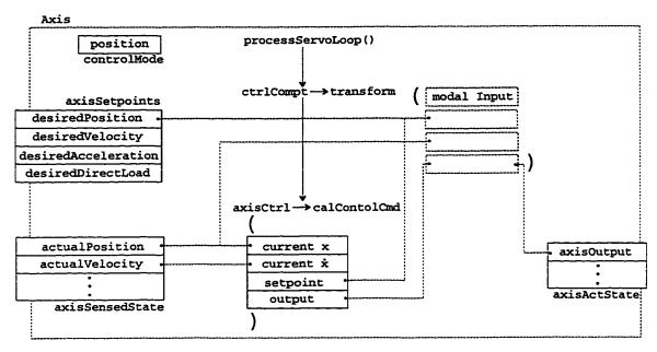
Figure 3.3: Object interactions in processing a servo loop
