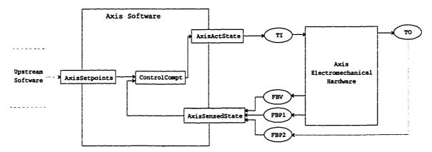
Figure 3.1: Overview of axis servo-control software model
