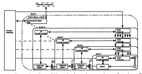
Figure A.2: Control hierarchy for an integrated manufacturing cell
