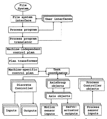
Figure 2.2: Data flow through an example configuration
