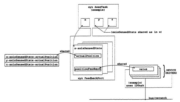
Figure 6.2: Efficient update of shared, yet encapsulated, objects in hard real-time control
