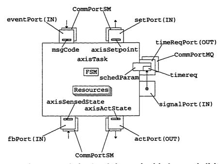
Figure 4.2: Structure of a hard real-time task with short periodicity — one-axis example
