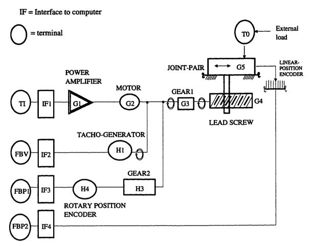
Figure 3.4: Schematic block diagram of a typical translational axis.
