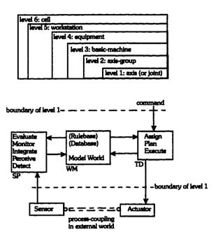
Figure A.1: Levels of control and tasks within a level
