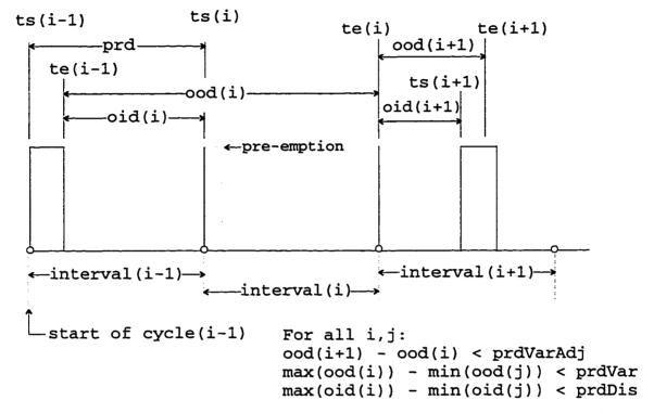
Figure 4.1: Specification of a period and time distance variation constraints
