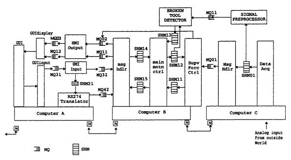
Figure 2.4: Schematic block diagram of a distributed control system testbed.
