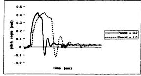
Figure 5.11: Aircraft pitch performance for different controller task levels.
