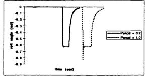
Figure 5.12: Aircraft roll performance for different controller task levels.
