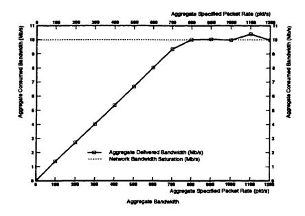
Figure 4.15: Network bandwidth saturation
