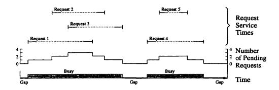
Figure 2.6: Measuring Utilization via Gap Estimation
