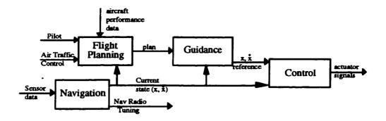
Figure 5.5: Flight management system functions.
