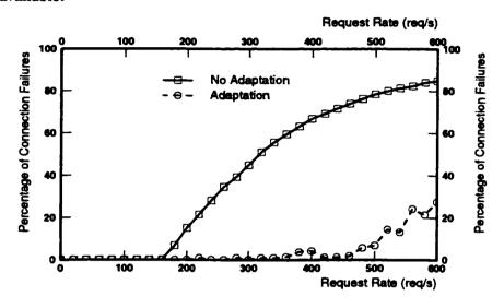
Figure 2.5: Adaptation and Connection Failure Probability
