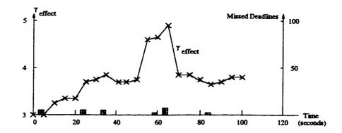
Figure 4.9: Improved responsiveness due to QoS level adjustment heuristic
