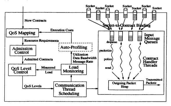
Figure 4.1: Communication subsystem architecture
