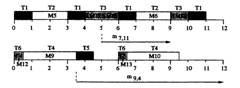
Figure 6.1: Computing message priority order  $Ord(V_{root})$ .
