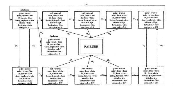
Figure 4-12: The State Diagram with All 7 Required Actions to Guarantee 100% Safety
