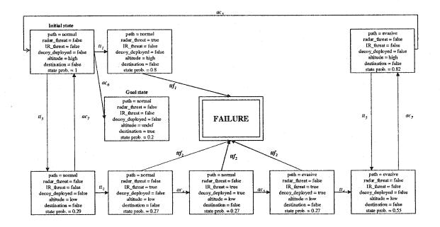
Figure 4-13: The State Diagram Ignoring the Radar Threat; Utility = 0.2
