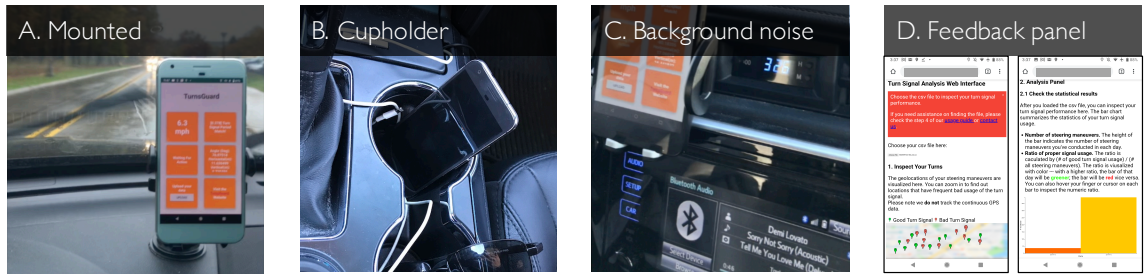
Figure 5.1: We designed, implemented and tested a smartphone-based tool (TurnsGuard) for profiling a driver’s inattentive steering maneuvers, i.e., turning or changing lanes without giving turn signals. A, B, and C demonstrate TurnsGuard’s robust performance under different usage contexts — mounted, cupholder, and under background noises (e.g., music), respectively. Please refer to our Video Figure to see how TurnsGuard works in the real-world. D shows the online feedback panel (elaborated in Sec. 5.4) for contextualizing the detection results and arousing the driver’s attention.
