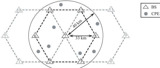
Fig. 4. An illustration of hexagonal BS deployment for dGA, from the view of BS 7 (the number in a BS is its BS index)
