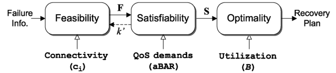
Fig. 3. Localized reconfiguration planning in ARS. ARS generates a reconfiguration plan by breaking down the planning process into three processes with different constraints.
