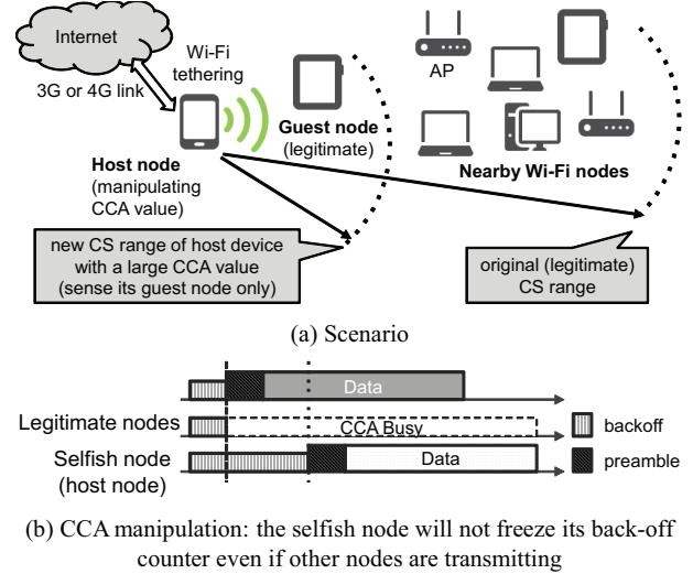
Fig. 1. Illustration of CCA threshold manipulation in Wi-Fi tethering.
