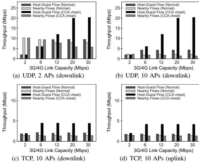
Fig. 2. Impact of selfish carrier sense on throughput of transport-layer protocols on 802.11g PHY/MAC over various 3G/4G link capacities and AP densities.
