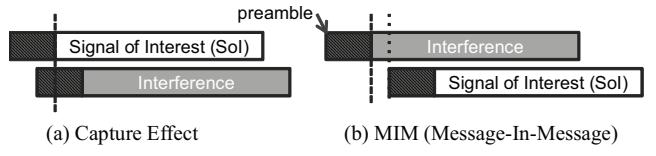
Fig. 3. Physical (PHY) capture and MIM: MIM-capable receiver can decode a strong signal of interest (SoI) even if it arrives later than the interference [5].
