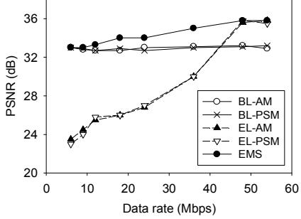
**Fig. 11. PSNR comparison with varying PHY data rate  $D$**
