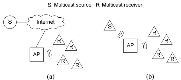
**Fig. 1. Multicast scenarios:** (a) traditional scenario; (b) target scenario (multicast within hotspot).
