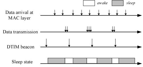
**Fig. 7. Packet transmission and reception timing of video sender and change of video sender's state with the sleep-scheduling module.**
