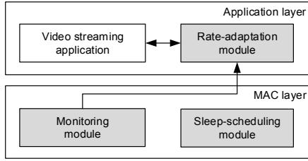
**Fig. 5. System architecture of EMS. Gray boxes are new module proposed in EMS.**
