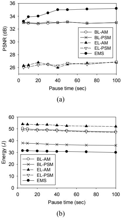
Fig. 14. Simulation results: Performance comparisons with varying pause time. (a) PSNR. (b) Consumed energy.
