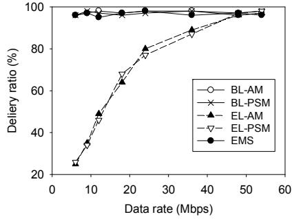
**Fig. 10. Delivery ratio comparison with varying PHY data rate  $D$**
