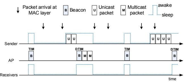
**Fig. 4. Ideal operation of multicast sender under PSM**
