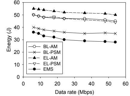
**Fig. 13. Consumed energy comparison with varying PHY data rate  $D$**
