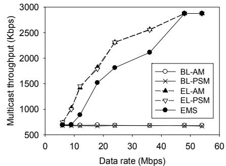
**Fig. 9. Multicast throughput comparison with varying PHY data rate  $D$**
