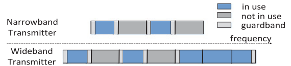
Fig. 3. The wideband and narrowband transmitters share spectrum chunks in a fine-grained (possibly discontinuous) manner.
