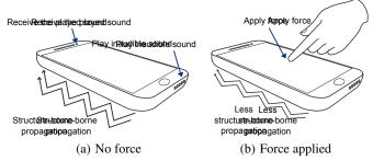
Figure 1—Structure-borne propagation and the applied force. When no force is applied to the phone, the frame and internal components of the phone can vibrate freely, and hence the played inaudible sound can easily propagate through the phone's body.
