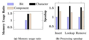
**Fig. 2:** On the granularity of trie-based structures. We use the performance of the bit-level trie as the baseline for the comparison. According to our evaluation results, we choose the character-level trie as the basis of NameTrie since it provides a more balanced trade-off than the other two alternatives.
