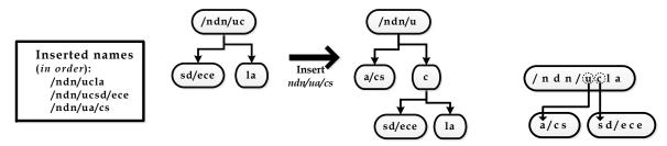
(a) Inserting /ndn/ua/cs in a conventional character-level trie, which causes node partitioning.
