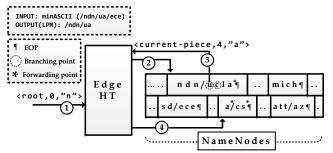
**Fig. 7:** Lookup of the name */ndn/ua/ece* in the NameTrie. For simplicity, characters are used instead of minASCII codes. *NameNodes* and *EdgeHT* have already stored the name pieces and their branching information according to Fig. 6.
