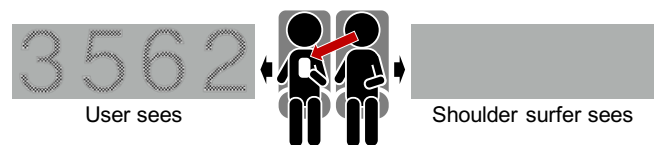
Figure 1: A common case of shoulder surfing in a train/bus and the effect of applying our proposed solution, HideScreen.
