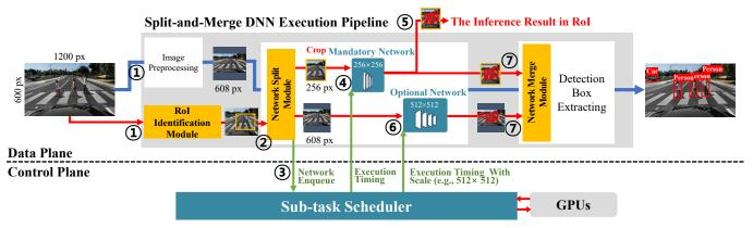
Fig. 4. System-level overview of DNN-SAM
