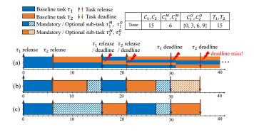
Fig. 5. Execution timeline of multiple DNN tasks under (a) Baseline, (b) EDF-MandFirst, and (c) EDF-Slack scheduling policies.
