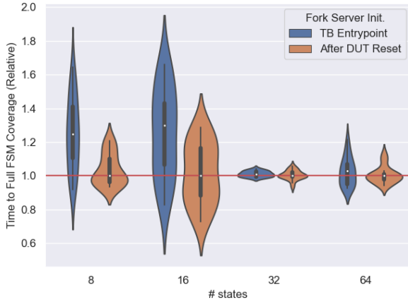
Figure 10: Hardware Resets vs. Fuzzer Performance. Fuzzing run times across across digital locks (similar to Fig. 8) with different fork server initialization locations in the testbench to eliminate overhead due to the repeated simulation of hardware DUT resets. DUT resets are only a fuzzing bottleneck when DUTs are small, reducing fuzzer–HSB integration complexity.
