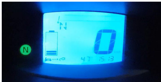
Fig. 20. Unsuccessful instance of the fabrication attack: the dashboard displays maximum driving range (47 km), but the original SoC.
