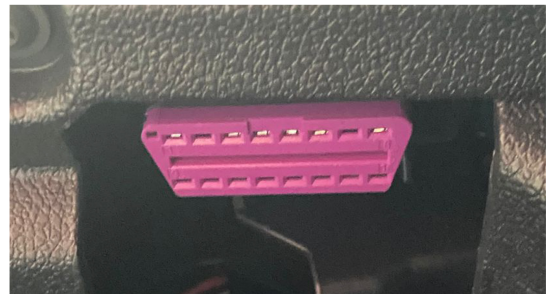
Fig. 8. OBD-II port in a Cupra Formentor, model year 2021.
