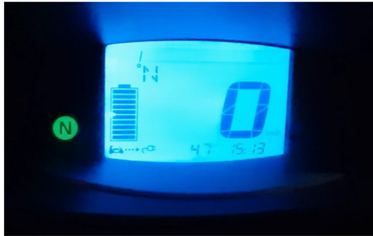
Fig. 19. Successful instance of the fabrication attack: the dashboard displays a full SoC and the maximum driving range (47 km).
