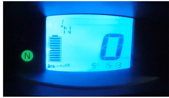
Fig. 21. Unsuccessful instance of the fabrication attack: the dashboard displays a full SoC, but the original remaining driving range (5 km).
