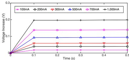
**Figure 11:** Voltage responses when charging a cell with different currents.
