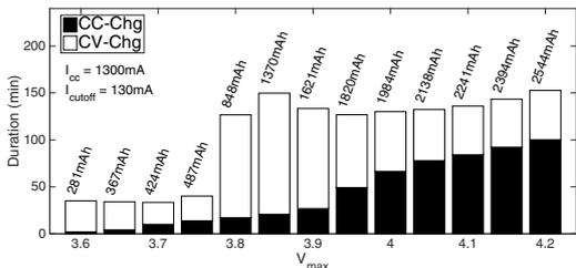
Figure 7: With CCCV, a smaller  $V_{\max}$  leads to less charged capacity but not necessarily a shorter charging time.
