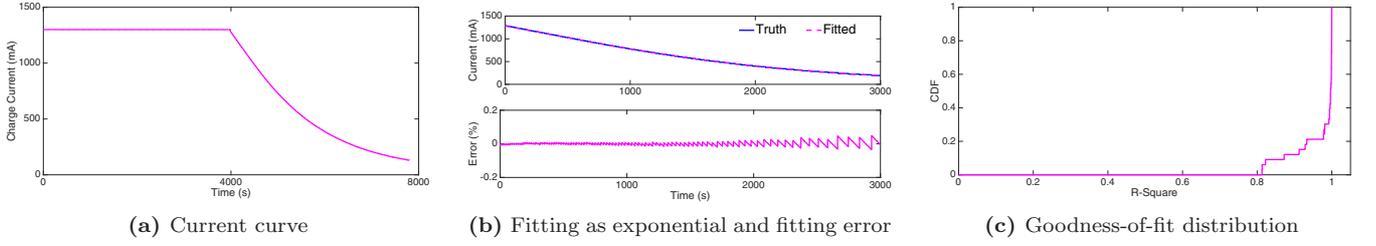
**Figure 15:** The charging current during CV-Chg fits a two-term exponential model.
