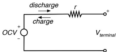
Figure 1: Circuit model of cells.
