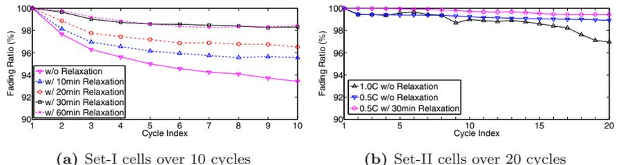
Figure 4: Insufficient relaxation leads to accelerated cell capacity fading.
