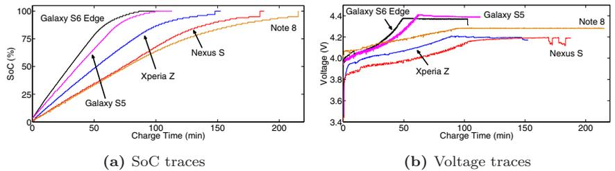
Figure 2: Charging processes of 5 mobile devices with respective chargers.
