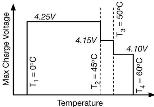
**Figure 14:** The maximum safe charge voltage of Lithium-ion cells with temperature [31].
