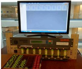
Figure 3: Battery tester and cells.
