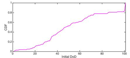
**Figure 13:** Mobile devices are often charged before completely discharged in most cases.
