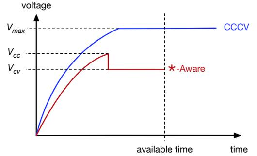
**Figure 9:** Illustration on the \*-AWARE-based charging process.
