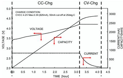
Figure 5: CCCV-based charging process [25].
