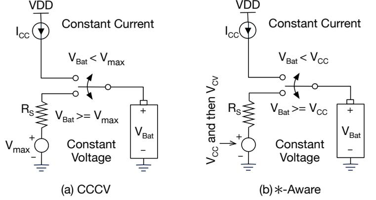
**Figure 17:** Implementation circuit schemata for CCCV and \*-Aware.
