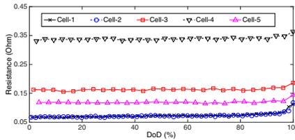
**Figure 12:** The cell resistance shows small variations throughout the charging process
